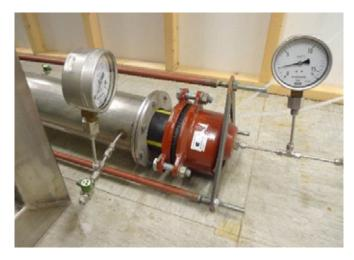
Figure 2. Permeation experimental setup in which the PE pipe (black with yellow stripes) is capped and pressurised whilst permeation is measured by gas chromatography in a stainless steel jacket pipe.
