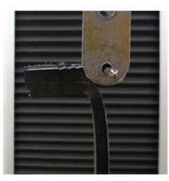
Figure 1. Peel test setup as per ISO 13954
